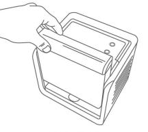
PLACE Place the water tank back onto the unit
